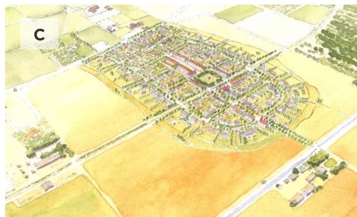
Cluster subdivision techniques are a key component of conservation development that preserves natural open space and productive agricultural lands. In the scenario above, a vacant 50+ acre tract of agricultural land (A) is subdivided into 225 single-family lots at a maximum of 10,000 acres per lot (B). The same development yield of 2.5 units per acre preserves a majority of the buildable acreage (C) where development standards rely on net density rather than lot size requirements.
