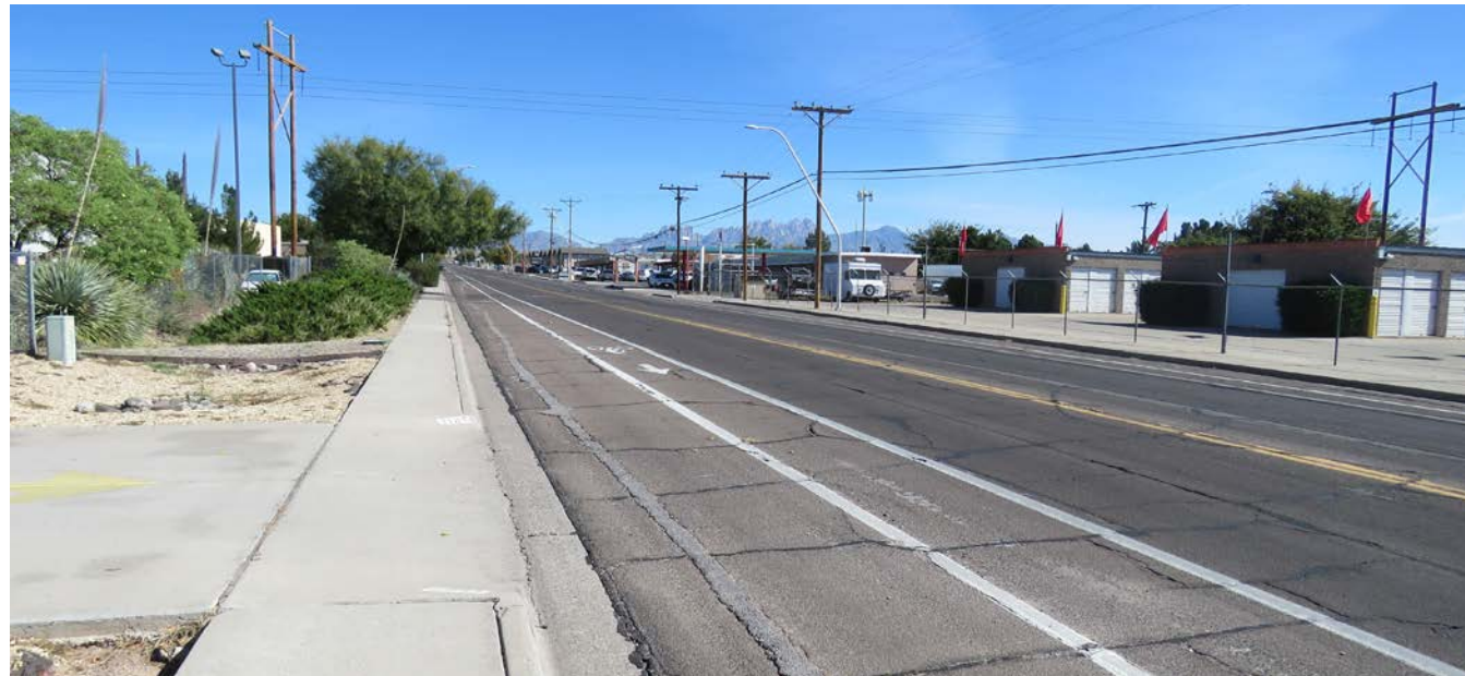
Madrid Avenue adheres to the City's Complete Streets policy by providing sidewalks, on-street parking, and bicycle lanes. The wide street cross-section does little to manage the speed of drivers. The street design and surrounding development patterns do not provide a design context which encourages bicycling, walking, or transit use.
