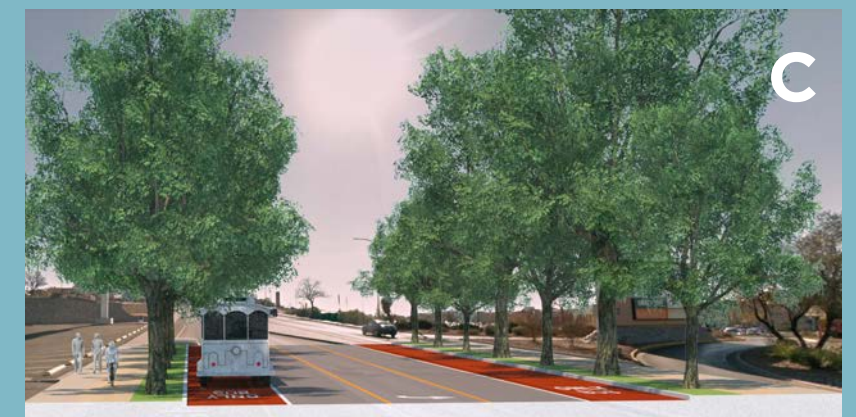
IMAGE C: The most popular option presented was the "Bus and Commuter Lanes" option. This option includes a dedicated lane for buses and commuters in each direction instead of parallel parking. This would encourage the use of buses and carpooling by making those options faster than a single occupancy car during rush hour.
