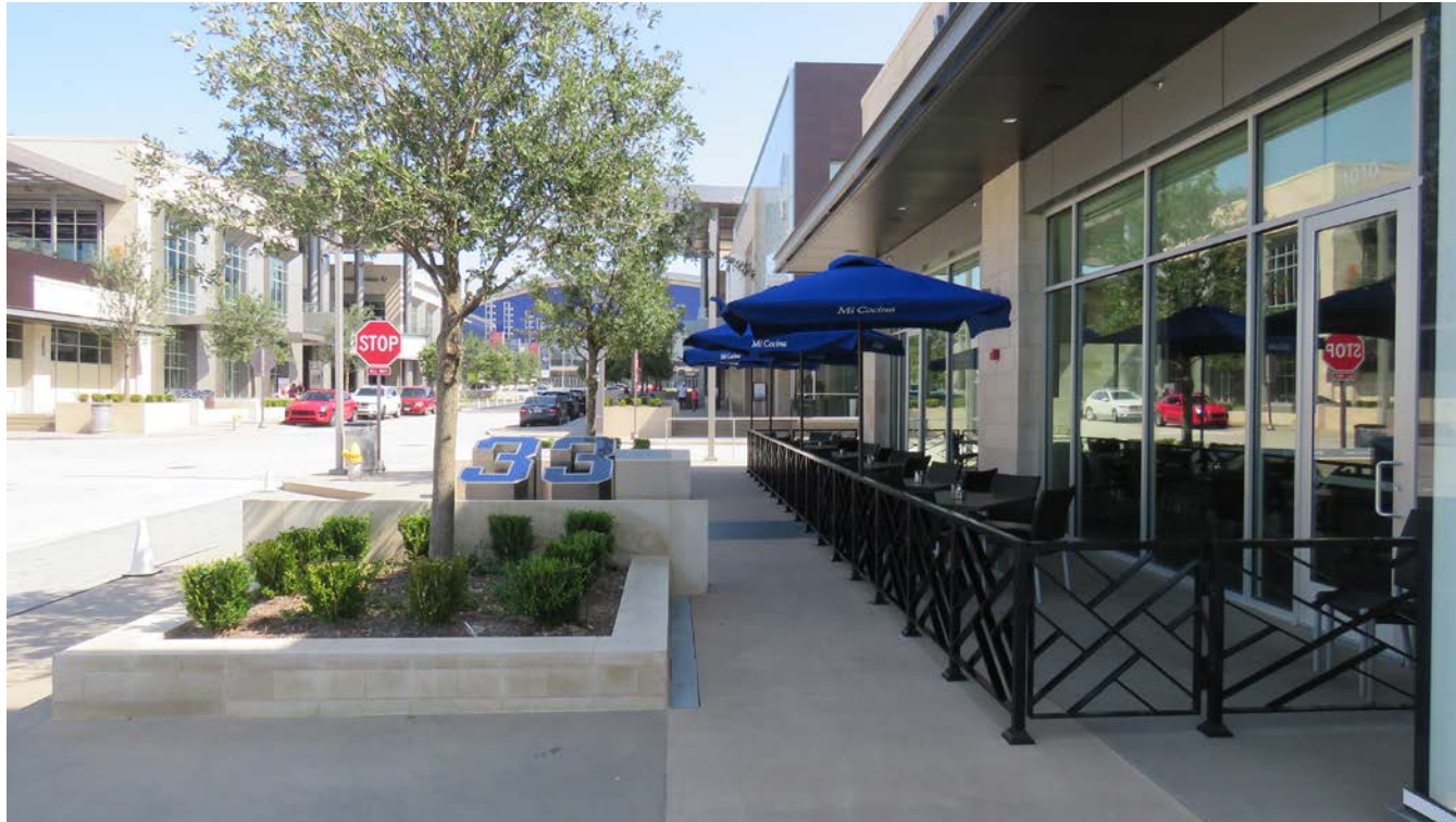
From left to right, active roadsides as a social space include an edge and furnishing zone, the thoroughway, and a frontage zone.
