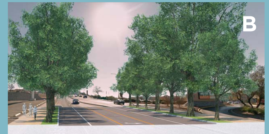
IMAGE B: This option shows a road diet to include street trees that separate car traffic from the sidewalk and a raised bike lane. Street trees provide shade and protection from vehicular traffic. These trees should be a drought-tolerant species that is naturally occurring in Las Cruces to minimize maintenance costs and increase the sustainability of the design.
