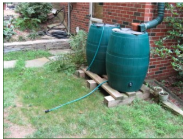
Cisterns and rain barrels are a cost-effective way to collect and store water for garden and lawn irrigation and would keep the water out of storm drains. Photos: www.epa.gov
