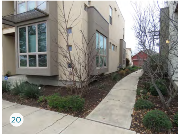
IMAGE 20: Pedestrian pathways should link streets at mid-block locations where the block length exceeds 600 feet.
