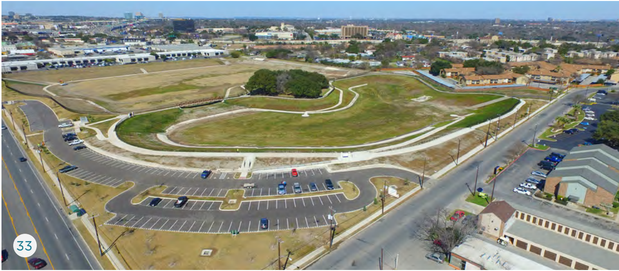
IMAGE 33: Storm Water detention facilities may be designed to provide extra multi-purpose field space. Laddie Place in San Antonio, Texas, currently allows for seven youth and/or two adult soccer fields.
