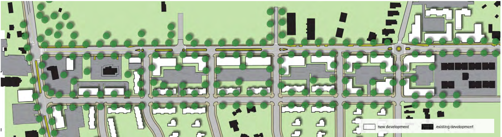
FIGURE II.8: The plan view of E. Madrid Avenue depicted above provides an example of how many of the streetscape enhancements depicted in Figure II.8 could be applied within a reconfigured corridor (as well as other optional traffic calming features). The figure also depicts possible building arrangements and roadway re-alignments that are consistent with the character area and character corridor development parameters (policies) that are recommended within other sections of the Blueprint.
