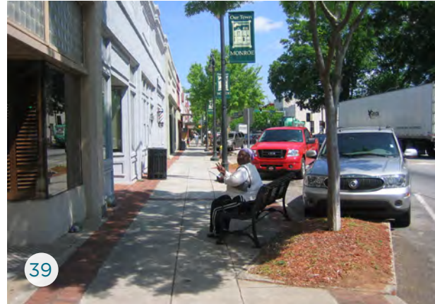
IMAGE 39: The frontage zone, through way, and furnishing zone are essential roadside elements that make urban streets comfortable and promote activity.
