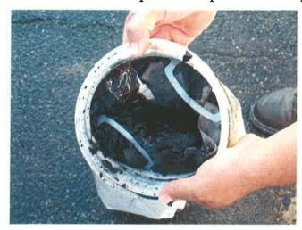
Another solution Utilities tested: NO-DES technology. NO-DES is a company that developed a process to run water between two fire hydrants at a very high velocity through very fine filters to filter out the minerals that discolor the water.
